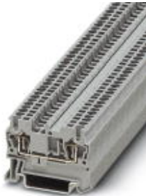
Feed-through terminal block, Connection method: Spring-cage connection, Cross section: 0.08 mm 2 - 1.5 mm 2 , AWG: 28 - 16, Width: 4.2 mm, Color: gray, Mounting type: NS 35/7,5, NS 35/15
