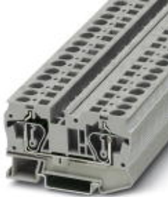
Spring-cage feed-through terminal block, Connection method: Spring-cage connection, Cross section: 0.2 mm 2 - 10 mm 2 , AWG: 24 - 8, Width: 8.2 mm, Color: gray, Mounting type: NS 35/7,5, NS 35/15
