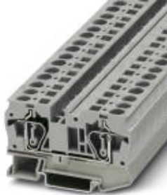
Feed-through terminal block, Connection method: Spring-cage connection, Cross section: 0.2 mm 2 - 10 mm 2 , AWG: 24 - 8, Width: 8.2 mm, Color: blue, Mounting type: NS 35/7,5, NS 35/15
