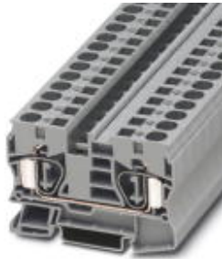
Feed-through terminal block, Connection method: Spring-cage connection, Cross section: 0.2 mm 2 - 16 mm 2 , AWG: 24 - 6, Width: 10.2 mm, Color: blue, Mounting type: NS 35/7,5, NS 35/15
