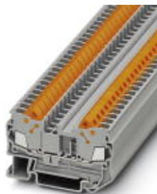
Feed-through terminal block, Connection method: Quick connection, Cross section: 0.5 mm 2 - 2.5 mm 2 , AWG: 20 - 14, Width: 6.2 mm, Color: gray, Mounting type: NS 35/7,5, NS 35/15
