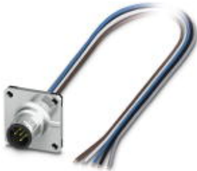
Sensor/Actuator flush-type plug, 5-pos., M12, A-coded, front/square flange mounting, with 0.5 m TPE litz wire, 5 x 0.34 mm 2
