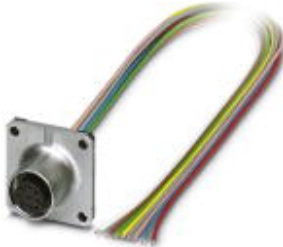
Sensor/actuator flush-type socket, 8-pos., M12, A-coded, front/square flange mounting, with 0.5 m TPE litz wire, 8 x 0.25 mm 2
