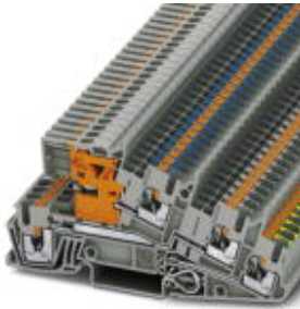
Installation level terminal block, Push-in connection, Cross section: 0.14 mm 2 - 4 mm 2 , AWG: 26 - 12, Width: 5.2 mm, Color: gray, Mounting type: NS 35/7,5, NS 35/15
