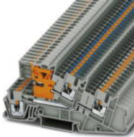
Installation level terminal block, Push-in connection, Cross section: 0.14 mm 2 - 4 mm 2 , AWG: 26 - 12, Width: 5.2 mm, Color: gray, Mounting type: NS 35/7,5, NS 35/15
