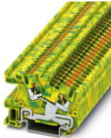
Installation terminal block, Push-in connection, Cross section: 0.14 mm 2 - 4 mm 2 , AWG: 26 - 12, Width: 5.2 mm, Color: green-yellow, Mounting type: NS 35/7,5, NS 35/15
