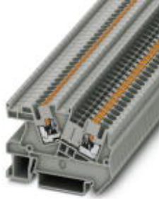
Installation terminal block, Push-in connection, Cross section: 0.14 mm 2 - 4 mm 2 , AWG: 26 - 12, Width: 5.2 mm, Color: gray, Mounting type: NS 35/7,5, NS 35/15
