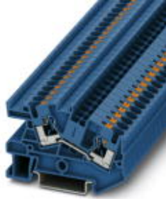
Installation terminal block, Push-in connection, Cross section: 0.2 mm 2 - 6 mm 2 , AWG: 24 - 10, Width: 6.2 mm, Color: blue, Mounting type: NS 35/7,5, NS 35/15
