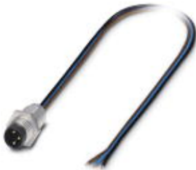
Sensor/actuator flush-type plug, 3-pos., M8, front/screw mounting, with M8 thread, with 0.5 m TPE litz wire, 3 x 0.25 mm²
