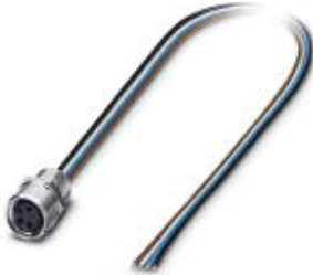
Sensor/actuator flush-type socket, 4-pos., M8, front/screw mounting, with M8 thread, with 0.5 m TPE litz wire, 4 x 0.25 mm 2
