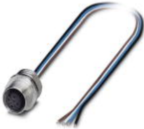
Sensor/Actuator flush-type socket, 4-pos., M12, A-coded, front/screw mounting with Pg9 thread, with 0.5 m TPE litz wire, 4 x 0.34 mm 2
