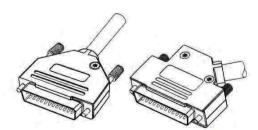
Complete the assembly by putting the second hood half over the assembly, and tighten with accompanied screw mounting set. Recommended Torque is 150 - 200 Ncm
