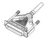
Place the assembly inside the metal cover.
