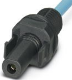
Photovoltaic connector, Nominal current: 27 A, Nom. voltage: 1500 V, Connection type: Crimp, Color: black, Can only be released using a tool
