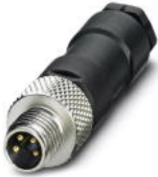
Sensor/actuator connector, male, straight, 4-pos., M8, solder connection, metal knurl, cable diameter max. 5 mm
