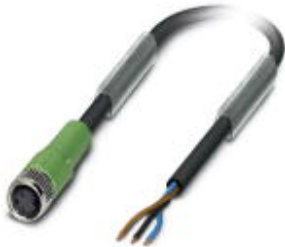
Sensor/Actuator cable, 3-position, PUR halogen-free, Black-gray RAL 7021, Free cable end, on Socket straight M8, Cable length: 3 m
