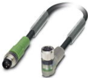
Sensor/Actuator cable, 3-position, PUR halogen-free, Black-gray RAL 7021, Plug straight M8, on Socket angled M8, with 2 LEDs, Cable length: 0.3 m
