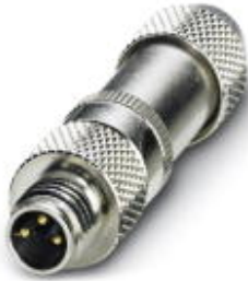
Sensor/actuator connector, male, straight, 3-pos., M8, shielded, solder connection, metal knurl, cable diameter max. 5 mm
