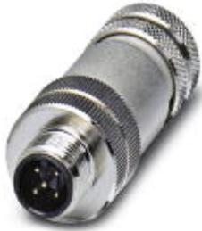
Sensor/actuator connector, male, straight, 5-pos., M12, shielded, A-coded, screw connection, metal knurl, cable screw connection Pg9
