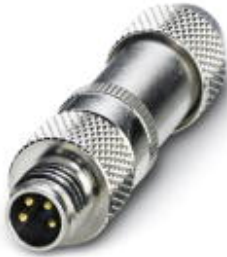
Sensor/actuator connector, male, straight, 4-pos., M8, shielded, solder connection, metal knurl, cable diameter max. 5 mm
