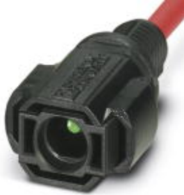
Photovoltaic connector, Nominal current: 40 A, Nom. voltage: 1500 V, Connection type: Crimp, Color: black, Can only be released using a tool
