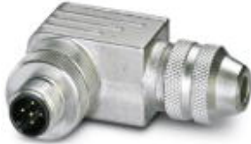
Sensor/actuator connector, male, angled, 5-pos., M12, shielded, A-coded, screw connection, metal knurl, cable screw connection Pg7
