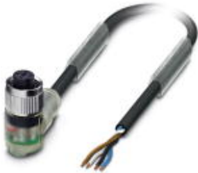
Sensor/Actuator cable, 4-position, PUR halogen-free, Black-gray RAL 7021, Free cable end, on Socket angled M12, A-coded, with 3 LEDs, Cable length: 10 m
