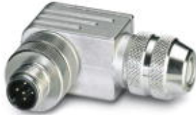
Sensor/actuator connector, male, angled, 5-pos., M12, shielded, A-coded, screw connection, metal knurl, cable screw connection Pg9
