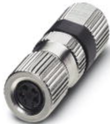
Sensor/actuator connector, female, straight, 4-pos., M8, Piercecon ® , metal knurl, cable diameter max. 5 mm
