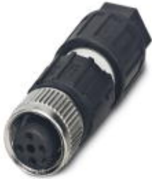
Sensor/actuator connector, 4-position, Socket straight M12, A-coded, Insulation displacement connection, Knurl material: Zinc die-cast, nickel-plated, External cable diameter 3.5 mm ... 6 mm
