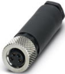
Connector, 4-position, Socket straight M8, A-coded, Screw connection, Knurl material: Nickel-plated brass, External cable diameter 3.5 mm ... 5 mm
