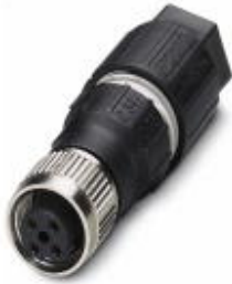
Sensor/actuator connector, 4-position, Socket straight M12, A-coded, Insulation displacement connection, Knurl material: Zinc die-cast, nickel-plated, External cable diameter 4 mm ... 8 mm
