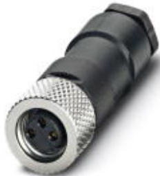
Sensor/actuator connector, female, straight, 3-pos., M8, solder connection, metal knurl, cable diameter max. 5 mm
