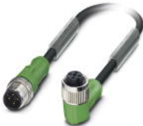
Sensor/Actuator cable, 4-position, PUR halogen-free, Black-gray RAL 7021, Plug straight M12, A-coded, on Socket angled M12, A-coded, Cable length: 3 m
