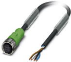
Sensor/Actuator cable, 4-position, PUR halogen-free, Black-gray RAL 7021, Free cable end, on Socket straight M12, A-coded, Cable length: 3 m
