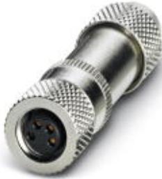
Sensor/actuator connector, female, straight, 4-pos., M8, shielded, solder connection, metal knurl, cable diameter max. 5 mm
