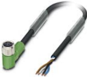
Sensor/Actuator cable, 4-position, PUR halogen-free, Black-gray RAL 7021, Free cable end, on Socket angled M8, Cable length: 5 m
