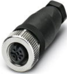
Sensor/actuator connector, female, straight, 4-pos., M12, A-coded, screw connection, metal knurl, cable screw connection Pg7
