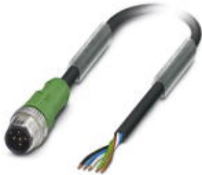
Sensor/Actuator cable, 5-position, PUR halogen-free, Black-gray RAL 7021, Plug straight M12, A-coded, on Free cable end, Cable length: 1.5 m
