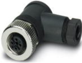
Sensor/actuator connector, female, angled, 4-pos., M12, A-coded, screw connection, metal knurl, cable screw connection Pg7
