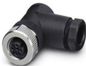
Sensor/actuator connector, female, angled, 5-pos., M12, A-coded, screw connection, metal knurl, cable screw connection Pg9
