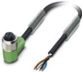
Sensor/Actuator cable, 4-position, PUR halogen-free, Black-gray RAL 7021, Free cable end, on Socket angled M12, A-coded, Cable length: 3 m
