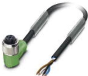
Sensor/Actuator cable, 4-position, PUR halogen-free, Black-gray RAL 7021, Free cable end, on Socket angled M12, A-coded, Cable length: 5 m
