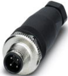
Sensor/actuator connector, male, straight, 4-pos., M12, A-coded, screw connection, metal knurl, cable screw connection Pg7
