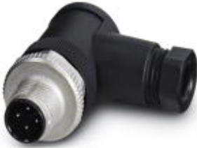
Sensor/actuator connector, male, angled, 4-pos., M12, A-coded, screw connection, metal knurl, cable screw connection Pg7
