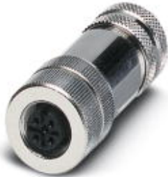
Sensor/actuator connector, female, straight, 5-pos., M12, shielded, A-coded, screw connection, metal knurl, cable screw connection Pg7
