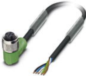
Sensor/Actuator cable, 5-position, PUR halogen-free, Black-gray RAL 7021, Free cable end, on Socket angled M12, A-coded, Cable length: 1.5 m
