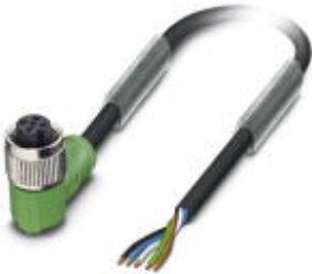
Sensor/Actuator cable, 5-position, PUR halogen-free, Black-gray RAL 7021, Free cable end, on Socket angled M12, A-coded, Cable length: 3 m
