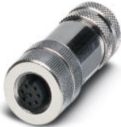
Sensor/actuator connector, female, straight, 8-pos., M12, shielded, A-coded, screw connection, metal knurl, cable screw connection Pg9
