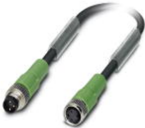
Sensor/Actuator cable, 3-position, PUR halogen-free, Black-gray RAL 7021, Plug straight M8, on Socket straight M8, Cable length: 1.5 m
