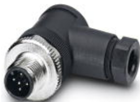
Sensor/actuator connector, male, angled, 5-pos., M12, A-coded, screw connection, metal knurl, cable screw connection Pg7
